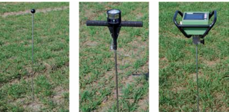
Instruments for measurement of the penetration resistance, from left to right: manual soil penetrometer, mechanical penetrometer, electronic penetrometer.
